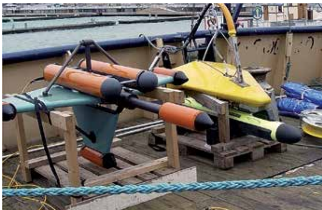
SEAQUEST MAGNETOMETER AND SIDE SCAN SONAR
